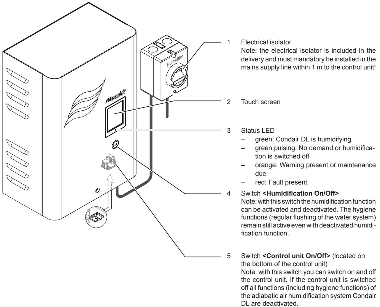
Abb. 7: Display and operating elements Condair DL
