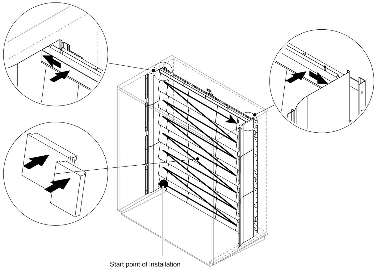
*Abb. 10: Installation of the ceramic plates*
